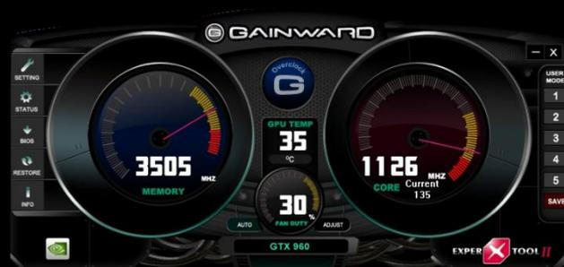
Gainward's Expertool II – the brand-new utility adds flexible fan curve control and BIOS saving feature for powerful GTX 960 Phantom GLH board.
