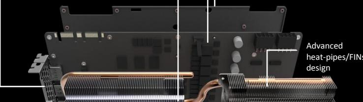
Advanced heat-pipes/FINs design
