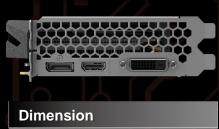
Board: 168mm(L)x126mm(W) Cooler : 2 slot Bracket: 2 slot Accessory 1. Manual
